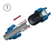
Pull up the nut, the clinching ring, the thrust ring, and O-ring on the pipe.
