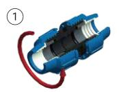
Limber up the nut, but do not remove it completely.
